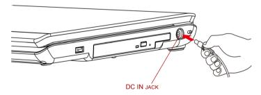
Figure 3-2 Connecting the adaptor to the computer
